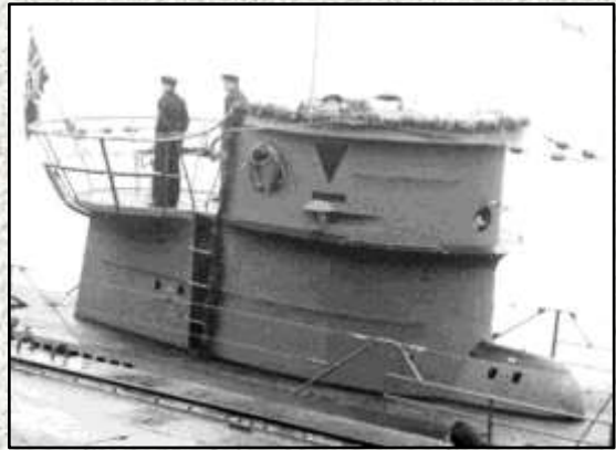
Above (6): The standard magnetic compass fairing on U 408. As the photo illustrates, the fairing abutted the front of the tower.
