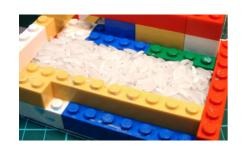
**Method 1 - Measurement:** use either water or uncooked rice. Though water is popular with casters, it is very messy and your mold and part must be dried thoroughly before pouring rubber. Rice is the cleanest and simplest method. Just buy a bag of cheap rice and keep it in your workshop in a plastic container. It's reusable! (Cooking the rice after is not recommended.)
