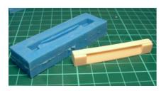
When the parts are cured, pop them out. They should come out easily, even parts with undercuts. The part may have flashing where resin spilled and created a thin skin. This can be sliced off after demolding, but it is important to at least lift the flash away from the rubber before demolding. Otherwise the rubber sticks and you can start tearing your mold. (Old molds that get stiff can be lightly baked in an oven at 120°C/250°F for four hours to revitalize.)
