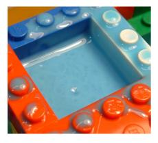
**TAPPING/VIBRATING:** Mix and pour, *then* worry about bubbles. Either constant tapping for a few minutes, or using something that vibrates, like a small palm sander or any motor that will shake the mold. Many report success. It can be violent to the mold, so some casters vibrate *before* pouring.
