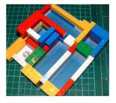
Lego Mold - 6 molds in one
