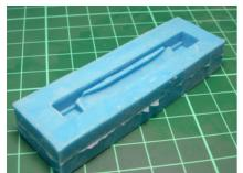
Suitable for any part that has at least one flat side with no detail, or a flat side that will never be seen on the finished work. The master is placed flat-side down on a base, then surrounded by a box. Rubber is poured over the part, filling the box. When cured, the base becomes the top, where resin will be poured. This is one of the most common molds in modelmaking.
