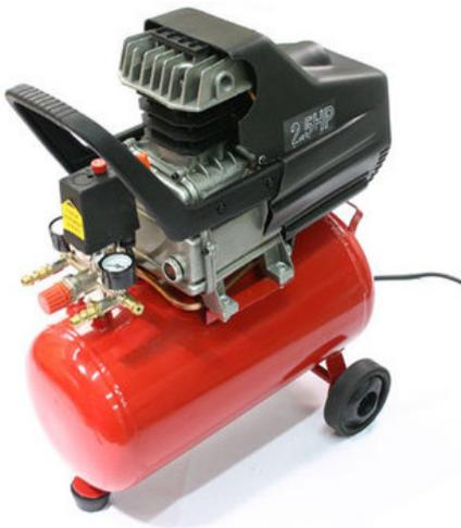
An airbrush/hobby compressor, one of the small 1/8<sup>th</sup> or 1/5<sup>th</sup> horsepower (hp) units, probably won't be big enough to do the job, but you can experiment before buying a bigger compressor. You need to pressurize the chamber smoothly, in about 10-20 seconds. Too fast might push resin out of molds, and too slow will let the resin kick before reaching full pressure.
